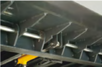
Reinforced self-cleaning hinges.
